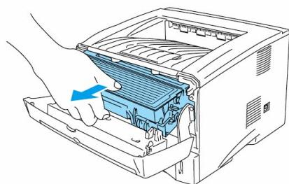
2. Pull out the drum unit assembly.
