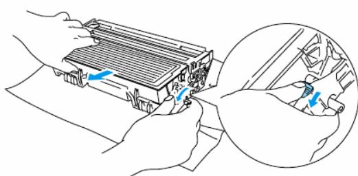
3. Push down the blue lock lever and take the toner cartridge out of the drum unit.
